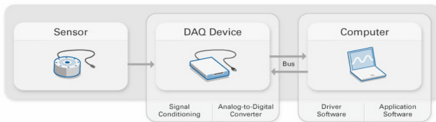
Fig. 1 – Block diagram of the DAQ system (Info. 1, ni.com).
